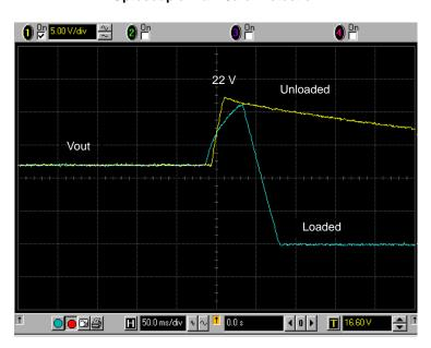
Figure 8. Fail-Safe Optocoupler Protection Triggered by a Short on the Secondary LED
